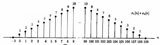
(b) The circular convolution,  $x_1[n]$  (100) $x_2[n]$ , can be obtained by aliasing the first 9 points of the linear convolution above:
